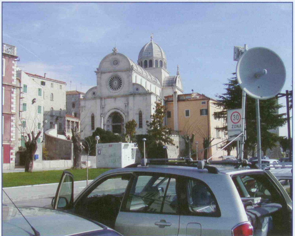
Above: A MICRO-LINK field test vehicle during RF measurements performed on WiMAX networks. Below: Anritsu's BTS Master is robust and comprises a wide range of functionalities
